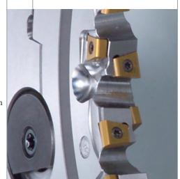
Pin milling cutter (Rough machining of the crank pin)
